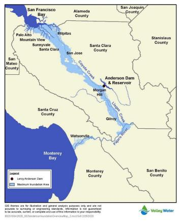
Maximum Flood Area from Anderson Dam Failure
